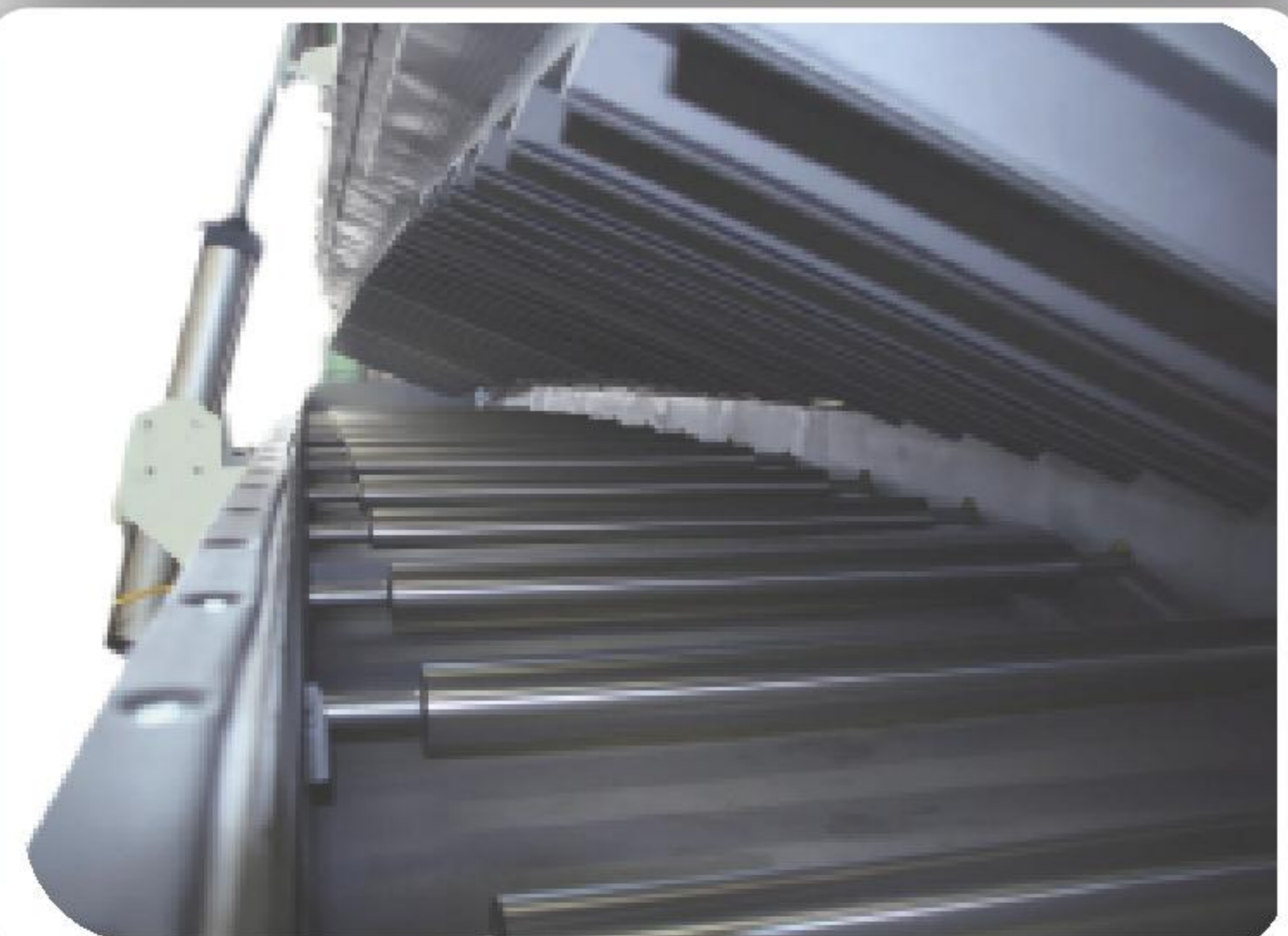
Drying tunnel guide rolls driven by motor
