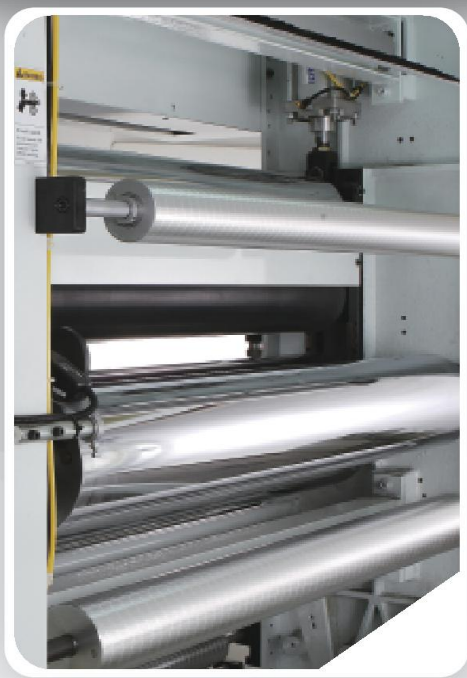
Three rolls laminating unit to keep well Pressure
