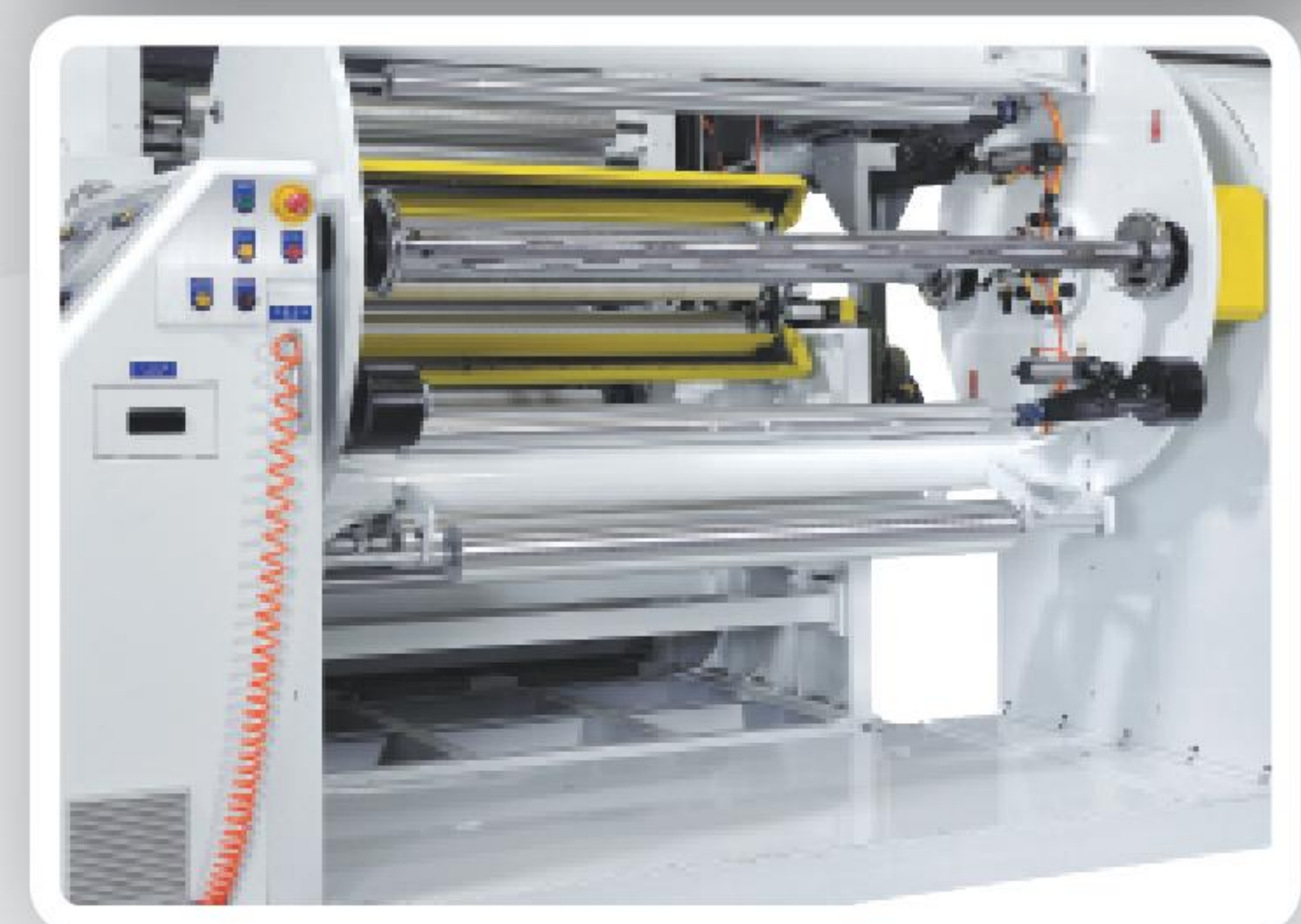
The speed of Ink furnisher roller can be adjusted as Auto/Manual
