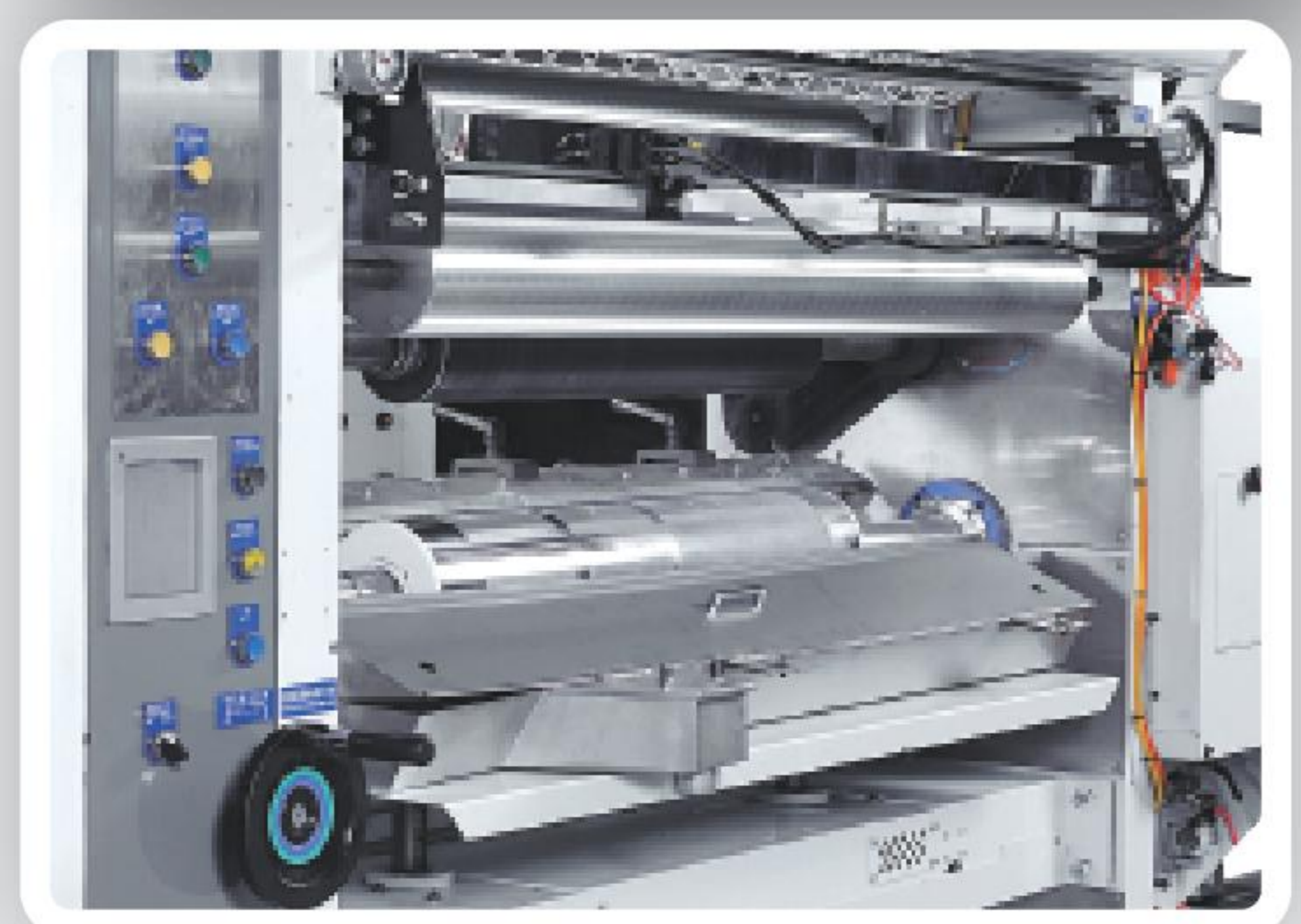
The speed of Ink furnisher roller can be adjusted as Auto/Manual
