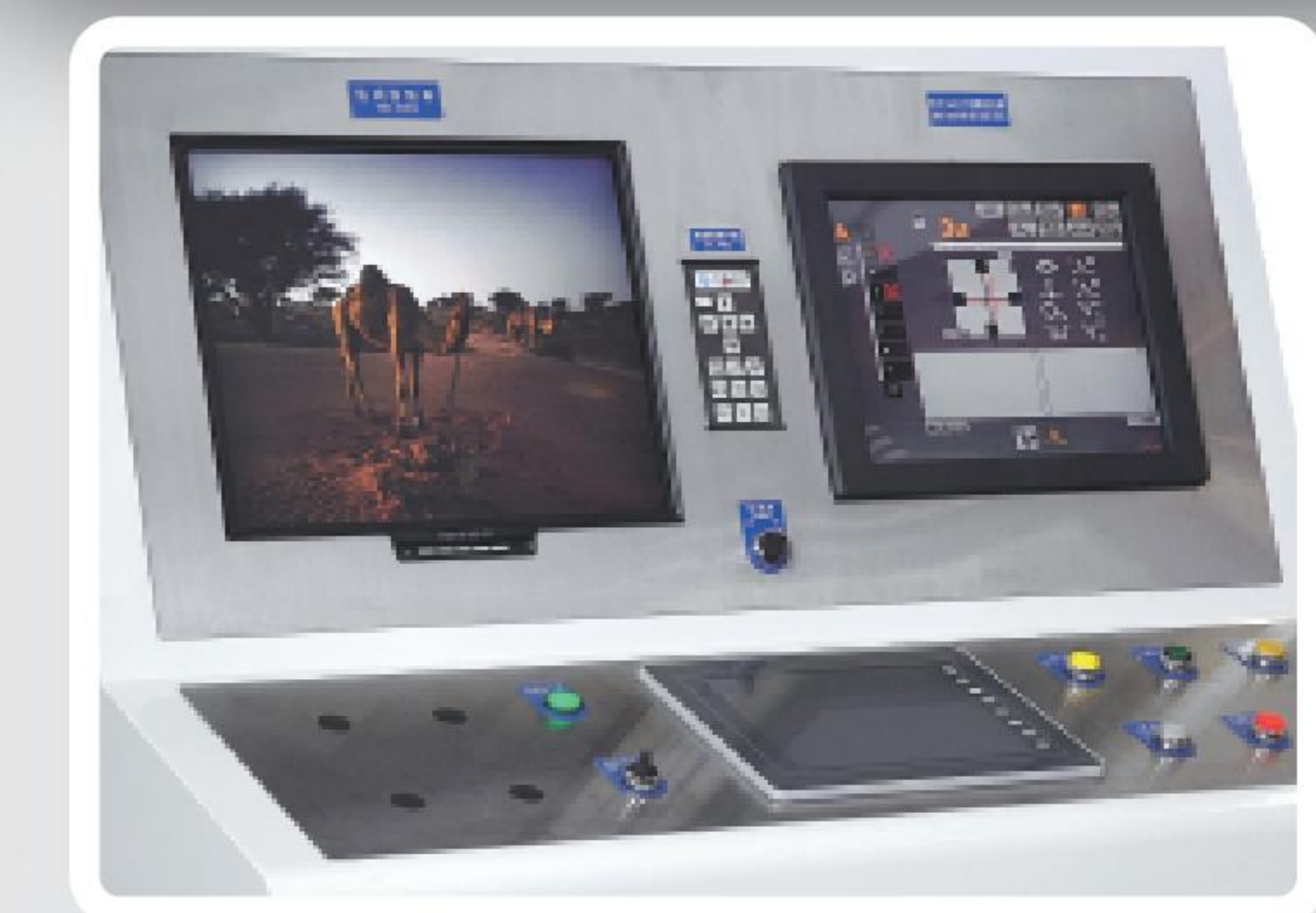
Integrated control panels managing operation, temperature, tension, printing registration..etc
